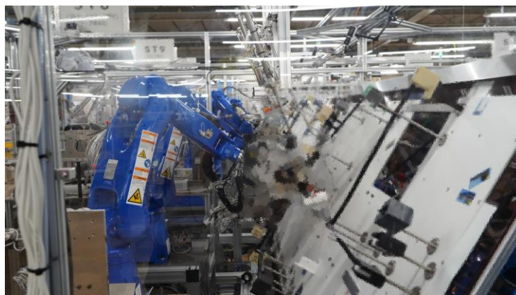
Automated wire harness production line at a Yazaki Corporation affiliate (Mine City, Yamaguchi Prefecture)
