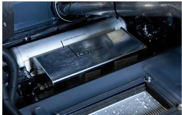
CO 2 capture device installed on the demonstration vehicle
