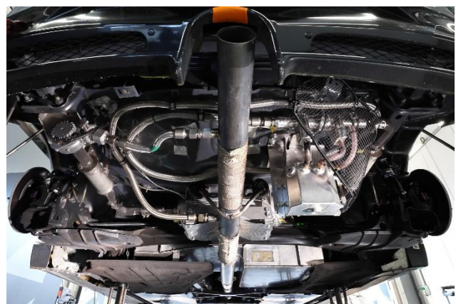
CO 2 capture device installed on the demonstration vehicle (Taken from the rear lower section of the vehicle)
