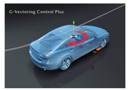
G-Vectoring Control Plus in operation (Mz: stabilizing moment; Fx: braking force)
